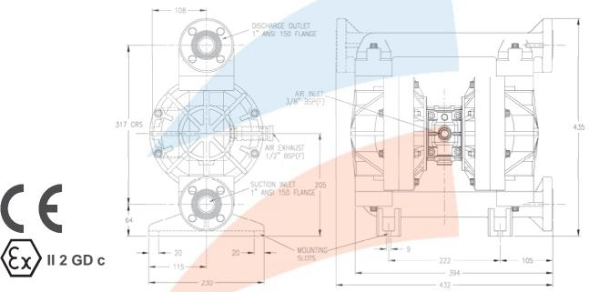
General Assembly: - B2505 Moulded Pump, all dimensions +/- 3mm
